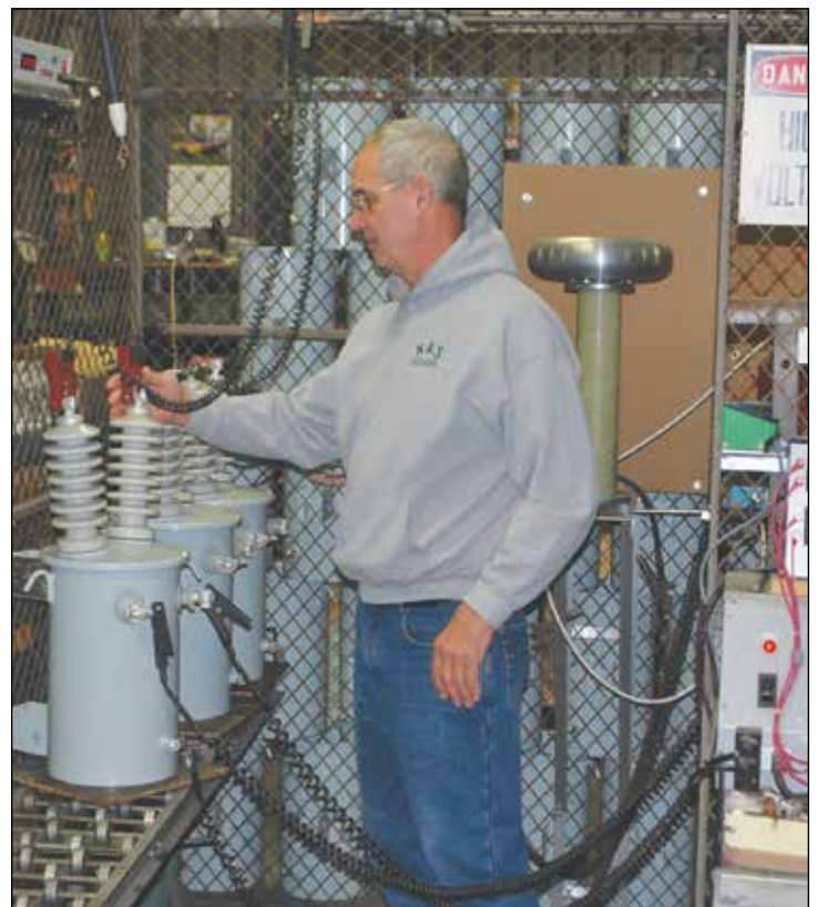
Gene Berman performing a final voltage test before the completed unit is shipped
