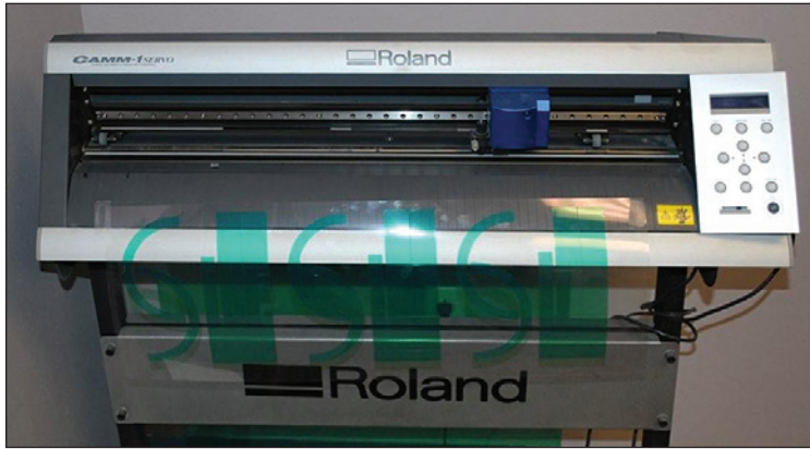
Roland die cut machine with custom designed masking
